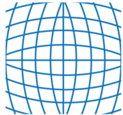
positive radial distortion "barrel"
